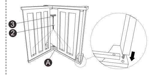
STEP 6: Invert the frame (step 4), fix the stretcher with STEP7: Place frame (step 6) to left legs(A), fix with bolt(1) and allen key(3).
