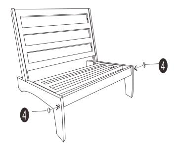
**STEP 8**: Fix the left end of stretcher with bolt(1) and allen key(3).
