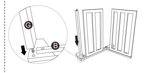
**STEP4**: Connect seat frame and back frame to right legs with bolt(2) and allen key(3).
