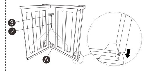
**STEP 6**: Invert the frame (step 4), fix the stretcher with bolt(1) and allen key(3).
